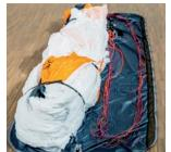
Stow the risers into the riser bag and place the lines into the SOFT-BAG
